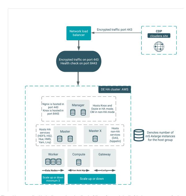
The architecture outlined in the diagram above handles the failure of one node in all of the host groups except for the "masterx" group. See the table below for additional details about the component interactions in failure mode:
