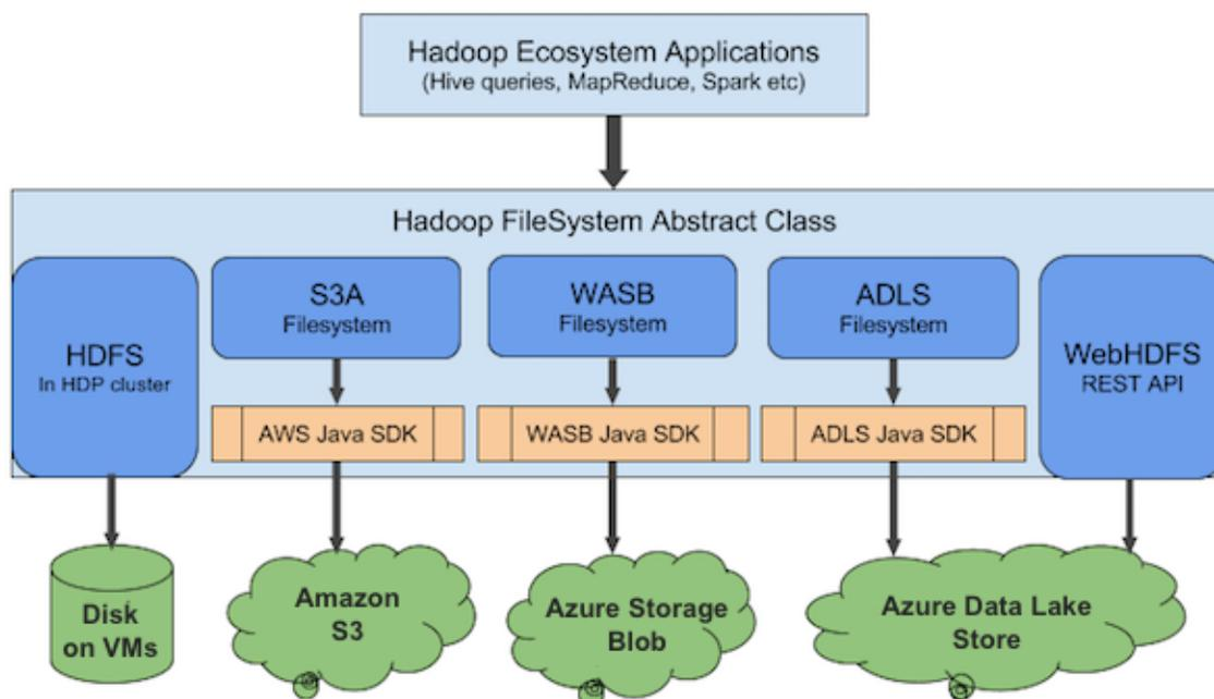
**Amazon S3** is an object store. The S3A connector implements the Hadoop filesystem interface using WWS Java SDK to access the web service, and provides Hadoop applications with a filesystem view of the buckets. Applications can seamlessly manipulate data stored in Amazon S3 buckets with an URL starting with the `s3a://` prefix.
