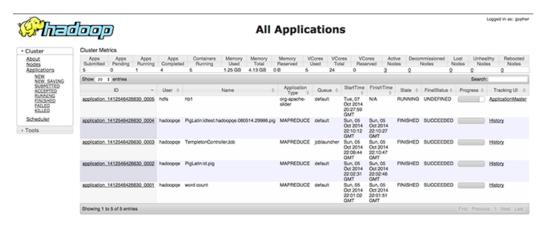
The specific information for the running application is accessible via the "ApplicationMaster" link that can be seen in the far right column of the row associated with the running application (probably the top row):
