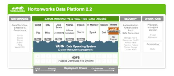
The core components of HDP are YARN and the Hadoop Distributed File System (HDFS).
