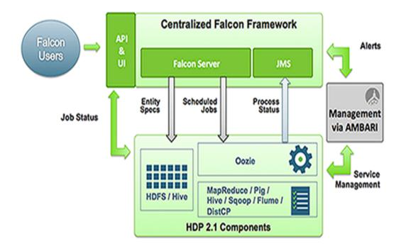
Falcon helps to address data governance challenges that can result when a data processing system employs hundreds to thousands of data sets and process definitions, using high-level reusable "entities" that can be defined once and reused many times. These entities include data management policies that are manifested as Oozie workflows.
