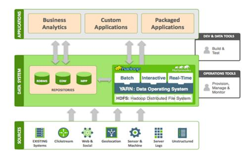
**HDFS** (storage) works closely with MapReduce (data processing) to provide scalable, faulttolerant, cost-efficient storage for big data. By distributing storage and computation across many servers, the combined storage resource can grow with demand while remaining economical at every size.
