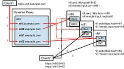
Routing rule example3 defined in nifi.properties (all nodes have the same routing configuration):
