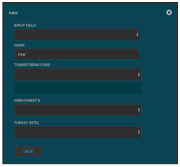
5. In the dialog box, enter the name of the new field in the NAME field, choose an input field from the INPUT FIELD box, and choose your transformation from the TRANSFORMATIONS field or enrichment from the ENRICHMENTS field.
