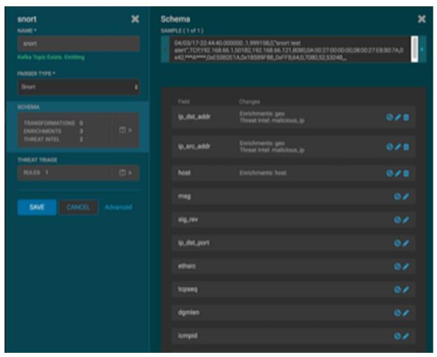
The Sample field, at the top of the panel, displays a parsed version of a sample message from the sensor. The Management UI will test your transformations against these parsed messages.
