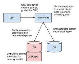
In this architecture, the NameNode is responsible for coordinating all of the DataNode off-heap caches in the cluster. The NameNode periodically receives a cache report from each DataNode. The cache report describes all of the blocks cached on the DataNode. The NameNode manages DataNode caches by piggy-backing cache and uncache commands on the DataNode heartbeat.
