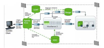
Typical Security Flow: Firewall, Routed Through Knox Gateway
