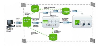
Typical Security Flow: Firewall, Routed Through Knox Gateway
