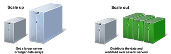
When individual hosts each possess a subset of the overall data set, the idea is for each host to work on their own portion of the final result independent of the others. In real life, it's likely that the hosts will need to communicate between each other, or that some pieces of data will be required by multiple hosts. This creates the potential for bottlenecks and increased risk of failure.
