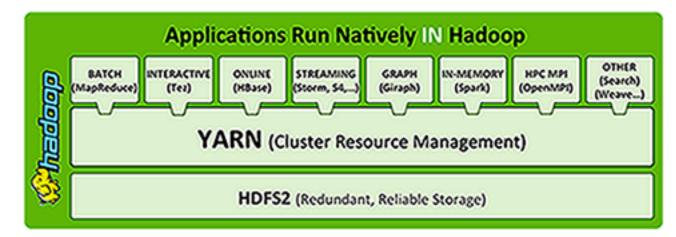
**HDFS** (storage) works closely with MapReduce (data processing) to provide scalable, faulttolerant, cost-efficient storage for big data. By distributing storage and computation across many servers, the combined storage resource can grow with demand while remaining economical at every size.
