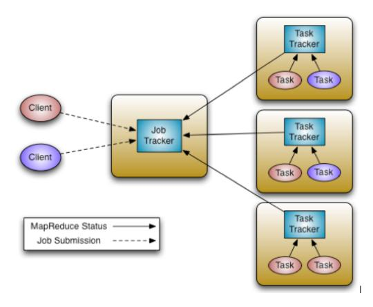
In Hadoop version 1, the Job Tracker is responsible for resource management (managing the worker nodes via the Task Trackers), tracking resource consumption and availability, and also job life-cycle management (scheduling individual tasks of a job, tracking progress, providing fault-tolerance for tasks, etc.).
