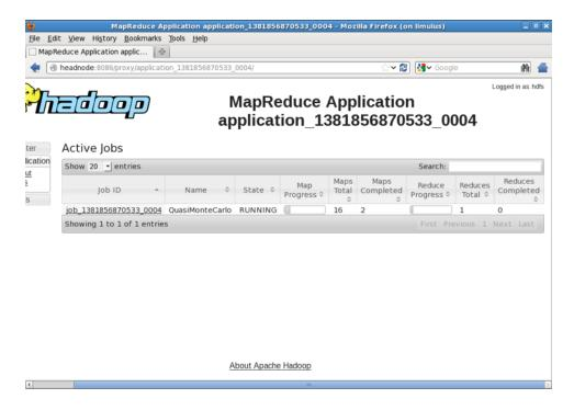
Details about the MapReduce process can be observed on the MapReduce Application page. Instead of Containers, the MapReduce application now refers to Maps and Reduces. Clicking the job\_138... link opens the MapReduce Job page:
