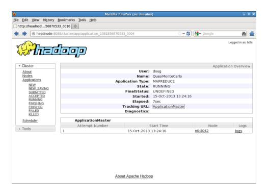
Clicking the **ApplicationMaster** link on the Application status page opens the MapReduce Application page shown in the following figure. Note that the link to the ApplicationMaster is also on the main Running Applications screen in the last column.
