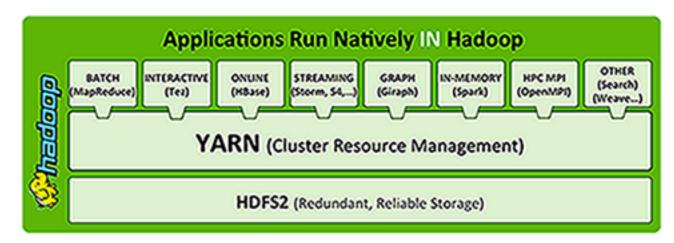
**HDFS** (storage) works closely with MapReduce (data processing) to provide scalable, fault-tolerant, cost-efficient storage for big data. By distributing storage and computation across many servers, the combined storage resource can grow with demand while remaining economical at every size.
