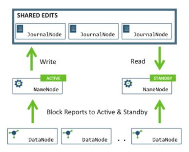
It is vital for the correct operation of an HA cluster that only one of the NameNodes should be Active at a time. Failure to do so, would cause the namespace state to quickly diverge between the two NameNode machines thus causing potential data loss. (This situation is called as **split-brain scenario**.)
