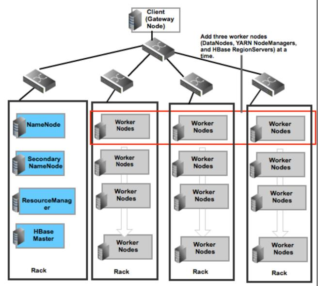
NOTE: DataNodes, NodeManagers, and RegionServers are typically co-deployed.
