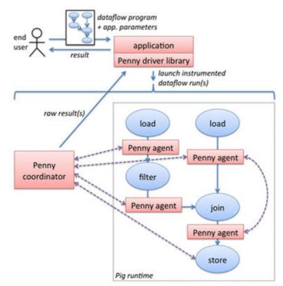
As shown in the diagram, Penny inserts one or more monitor agents (called "Penny agent" in the diagram) between steps of the Pig script, which observe data flowing between the Pig script steps. Monitor agents run arbitrary Java code as needed for your tool, which has access to some primitives for tagging records and communicating with other agents and with a central coordinator process (called "Penny coordinator" in the diagram). The coordinator also runs arbitrary code defined by your tool.
