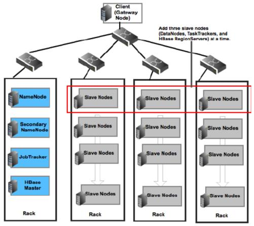
NOTE: DataNodes, TaskTrackers, and RegionServers are typically co-deployed.
